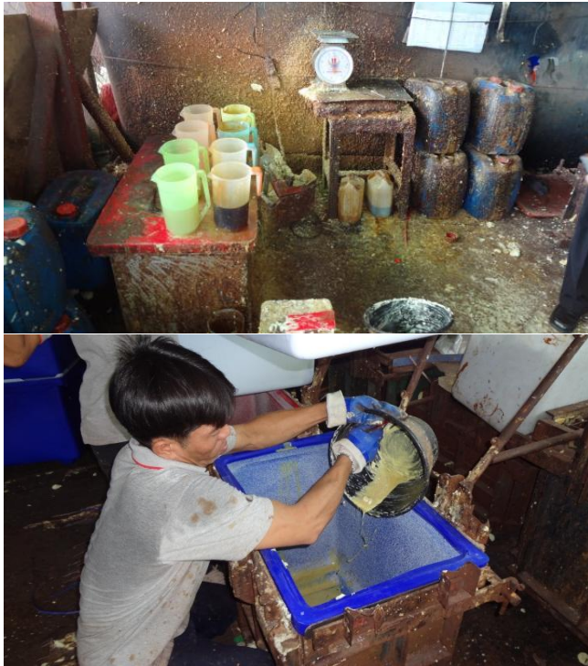
Photo-A-1 Top- Working condition manual mixing station. A portable electrical powered grinder which has been used for stirring the mixture before pouring into the mold.
